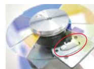
Magnetic sensor is strong against dust.
